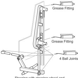
Steering with steering wheel and cover removed for clarity
