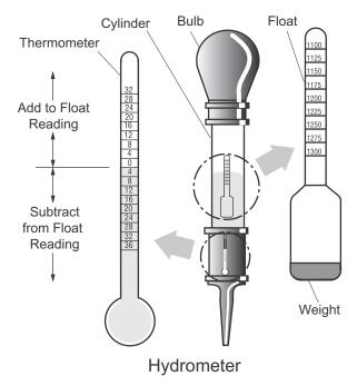
of water. A fully charged battery will test at 1.275 - 1.280 while a discharged battery will read in the 1.140 range.
