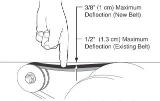
Fig. 11 Checking Belt Tension with Finger
