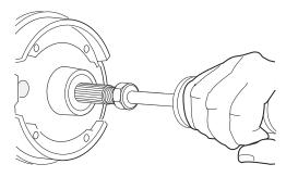
Fig. 4 Removing/Installing Axle Shaft
