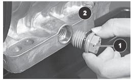
Fig. 5 Oil Drain Plug
