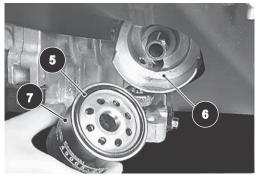
Fig. 7 Inspect Oil Filter
