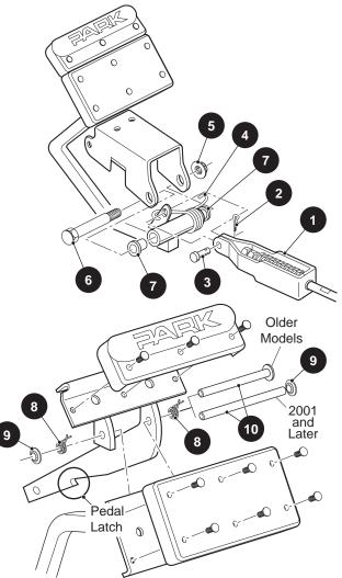
Fig. 27 Brake Pedal Removal and Installation.
