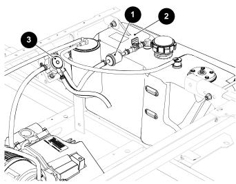
Fig. 9 Fuel Lines and Filter
