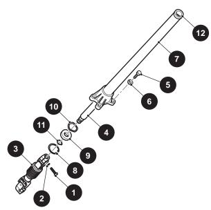
Fig. 24 Steering Shaft and Column
