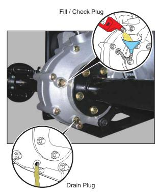
Fig. 2 Add, Check and Drain Rear Axle Lubricant
