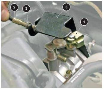
Fig. 4 Choke Cable and Housing
