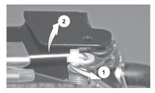
Fig. 6 Throttle Rod Removal
