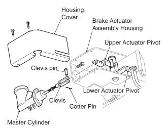
Fig. 1 Master Cylinder Replacement.
