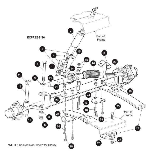
Fig. 7 Front Suspension Components
