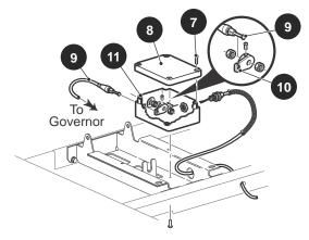
Fig. 5 Accelerator Cable at Pedal Box
