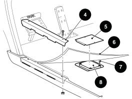
Fig. 4 Pedal Box Access
