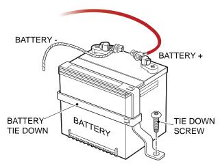
Fig. 1 Battery Removal
