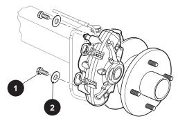
Fig. 17 Removing Brake Caliper
