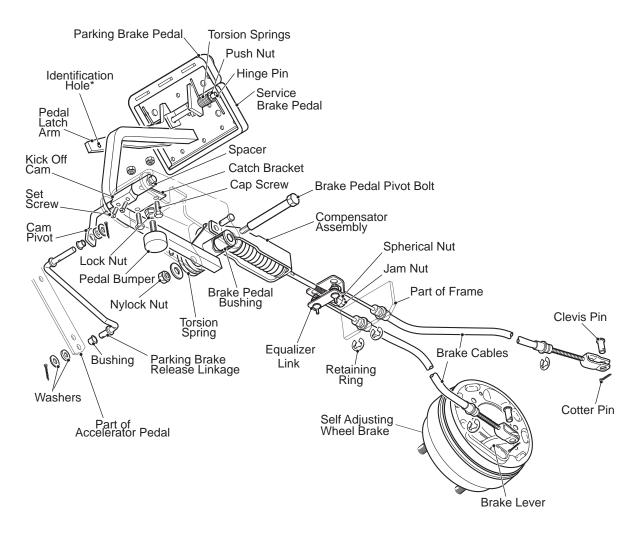
Fig. 1 Mechanical Brake System
