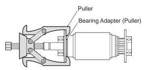
Fig. 9 Bearing Removal
