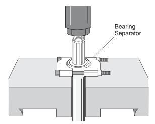
Fig. 5 Pressing Bearing from Axle Shaft
