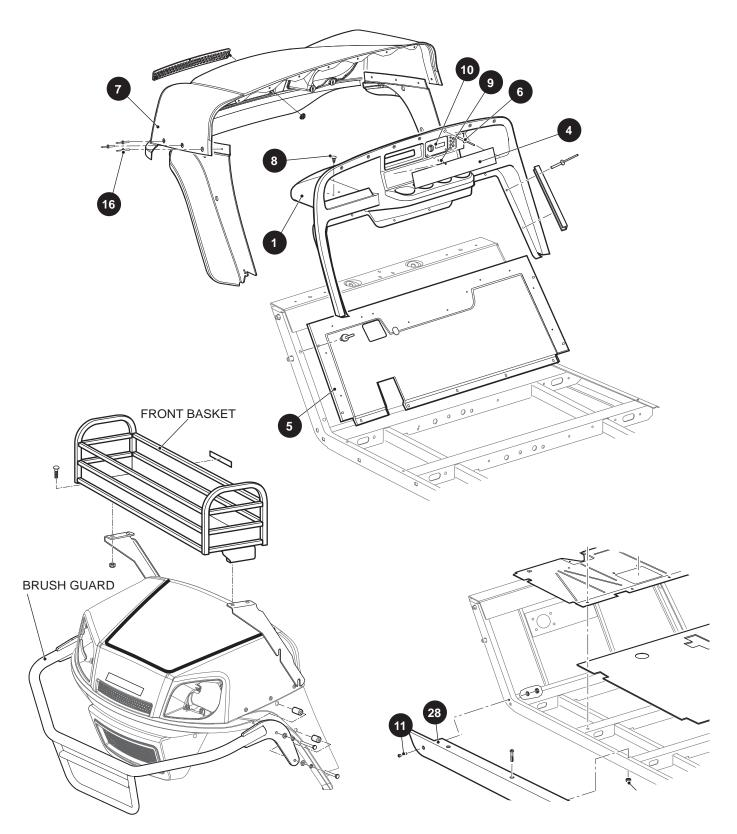
Fig. 2 Body Components (Front)
