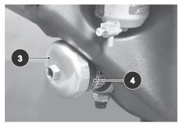
Fig. 6 Remove Oil Filter
