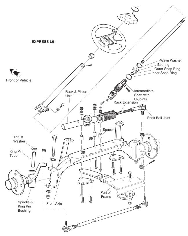
Fig. 1 Axle Mounted Steering and Front Suspension
