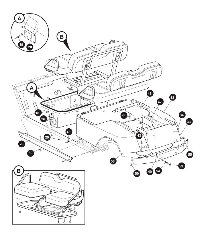
Fig. 3 Body Components (Seats and Rear)
