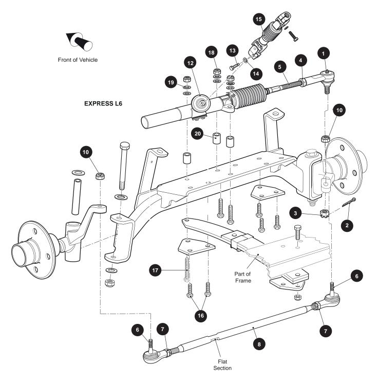
Fig. 12 Steering Components
