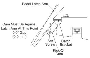
Fig. 12 Kick-off Cam Inspection Periodic Brake Performance Test (PBPT)
