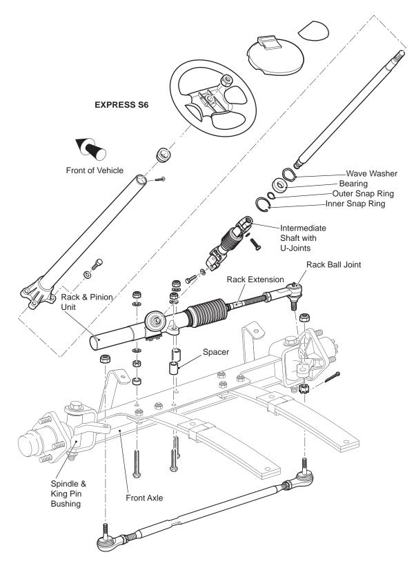
Fig. 2 Axle Mounted Steering and Front Suspension
