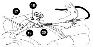
Fig. 7 Throttle Rod Adjustment
