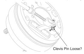
Fig. 19 Check Clevis Pins.
