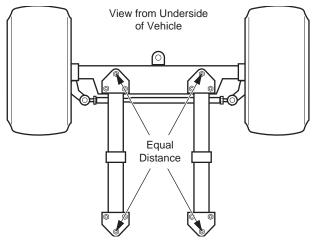
Fig. 8 Front Axle Alignment
