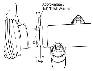
Fig. 21 Checking Gap
