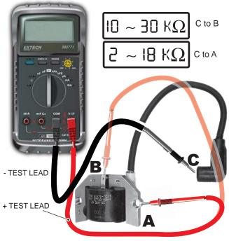
Fig. 6 Resistance Between C - B and C - A
