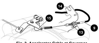
Fig. 3 Accelerator Cable at Governor
