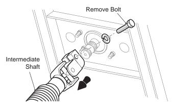
Fig. 6 Disconnect Intermediate Shaft to Center Steering Wheel
