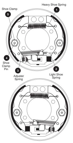
Fig. 24 Brake Shoes and Springs
