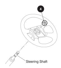
Fig. 23 Steering Wheel Replacement
