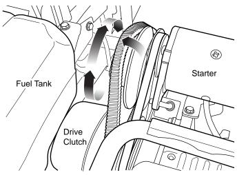
Fig. 2 Removing the Drive Belt
