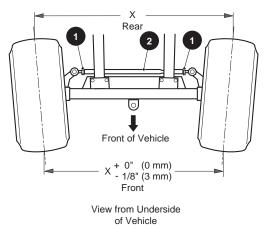
Fig. 5 Wheel Alignment
