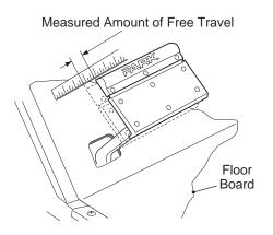
Fig. 9 Checking for Excessive Free Travel
