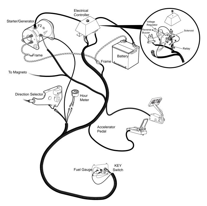
Fig. 3 Electrical System (Physical Location)
