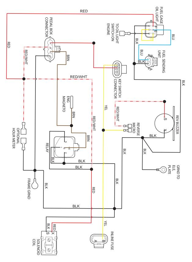
Fig. 1 Electrical System Wiring Diagram
