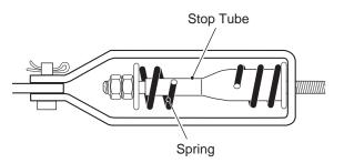
Fig. 4 Compensator Assembly
