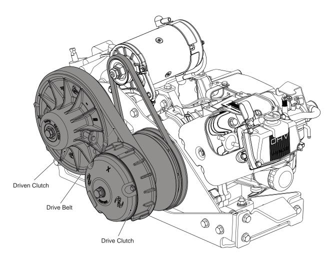
Fig. 1 Continuously Variable Transmission System (CVT)
