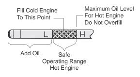
Fig. 2 Check Oil Level on Dipstick
