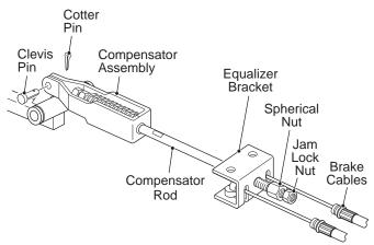
Fig. 26 Brake Cable, Equalizer and Compensator
