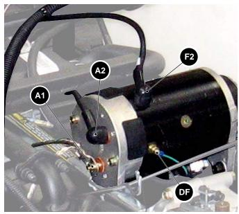
Fig. 14 Starter/Generator Wire Connections
