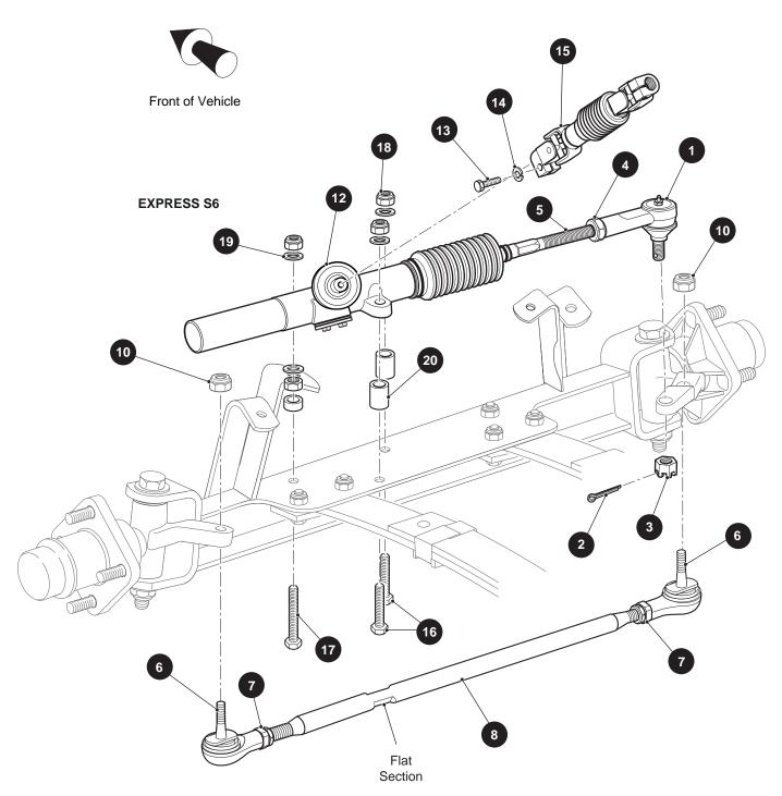
Fig. 12 Steering Components
