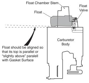
Fig. 7 Float Adjustment
