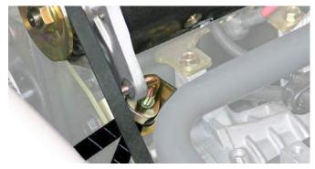
Fig. 13 Adjusting the Belt Tension
