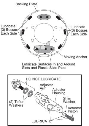
Fig. 22 Wheel Brake Lubrication Points
