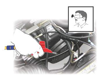
Fig. 16 Cleaning Cooling System with Air
