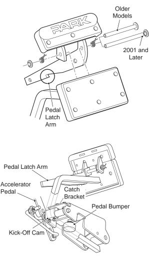
Fig. 3 Parking Brake and Kick-Off Mechanism
