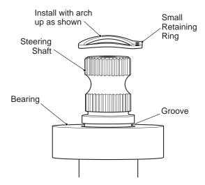
Fig. 25 Small Retaining Ring Orientation
