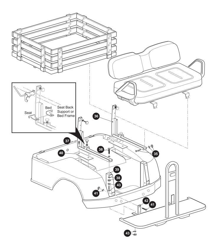
Fig. 4 Body Components (Cargo Box and Seat Foot Rest)
