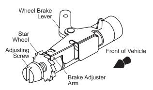
Fig. 15 Adjuster Mechanism
