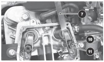
Fig. 21 Valve Clearance Adjustment
