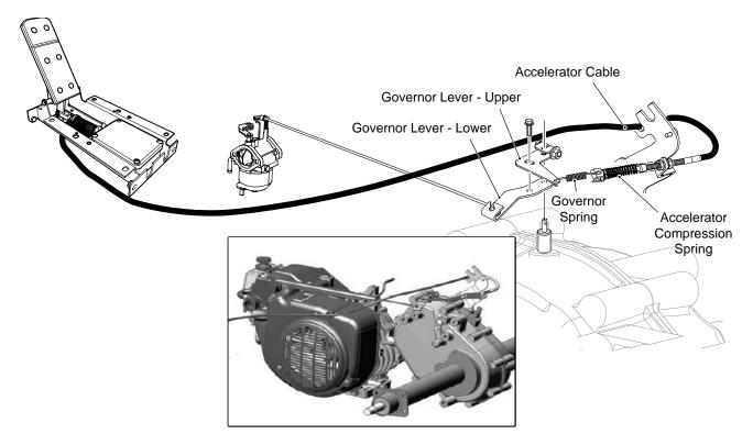
Fig. 1 Accelerator and Speed Control System
