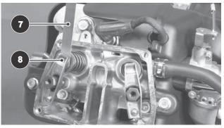
Fig. 20 Measure Valve Clearance
