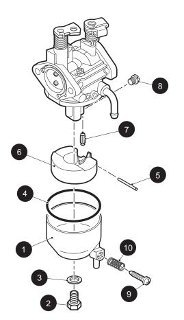
Fig. 6 Carburetor Disassembly
