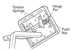
Fig. 11 Parking Brake Pedal Hinge Inspection
