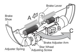
Fig. 2 Wheel Brake Adjustment
