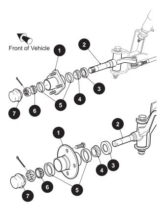
Fig. 11 Wheel Bearing Replacement
