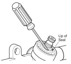
Fig. 16 Pinion Seal Replacement
