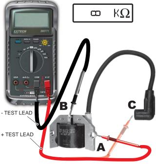
Fig. 5 Resistance Between B - A and B - C
