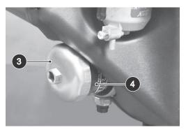
Fig. 6 Remove Oil Filter
