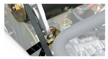
Fig. 13 Adjusting the Belt Tension
