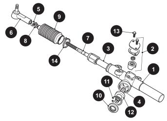
Fig. 19 Rack and Pinion Unit Disassembly
