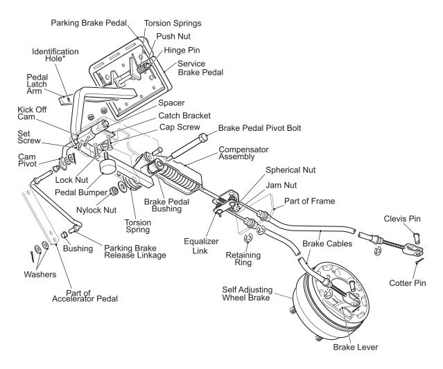
Fig. 1 Mechanical Brake System
