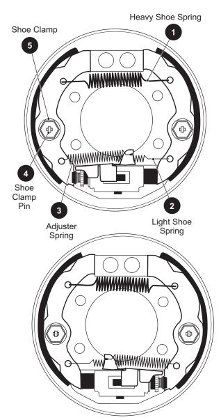
Fig. 23 Brake Shoes and Springs
