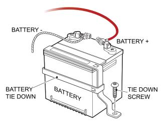
Fig. 1 Battery Removal
