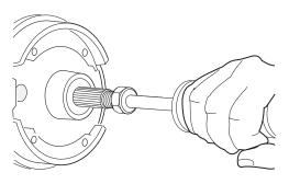
Fig. 4 Removing/Installing Axle Shaft
