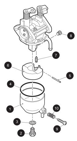
Fig. 6 Carburetor Disassembly
