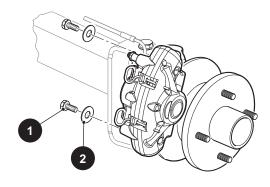
Fig. 17 Removing Brake Caliper
