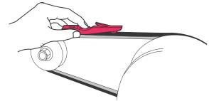
Fig. 10 Checking Belt Tension with Gauge
