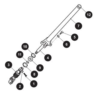
Fig. 24 Steering Shaft and Column
