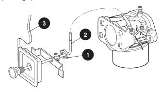
Fig. 7 Choke Cable Removal
