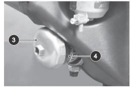
Fig. 6 Remove Oil Filter
