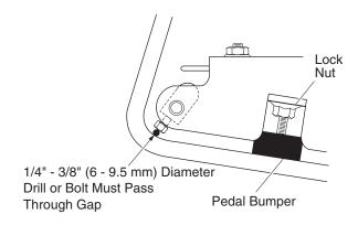
Fig. 28 Pedal Bumper Adjustment
