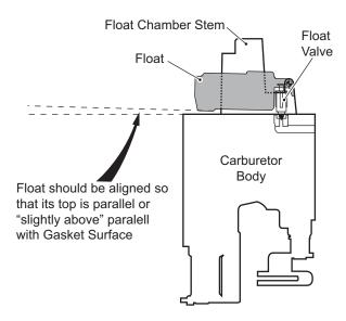
Fig. 7 Float Adjustment
