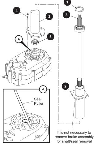
Fig. 6 Removing/Installing Seal
