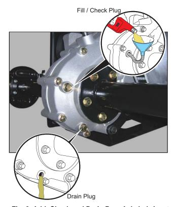
Fig. 2 Add, Check and Drain Rear Axle Lubricant
