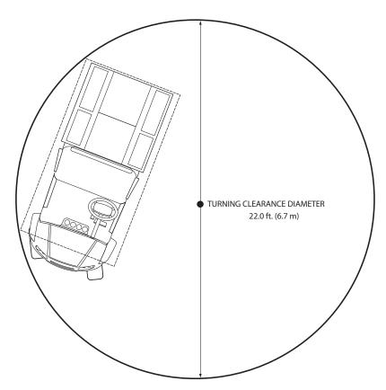
Fig. 6 Refresher Vechicle Dimensions, Incline Specifications and Turning Clearance Diameter
