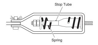
Fig. 4 Compensator Assembly Kick-Off Actuating Linkage
