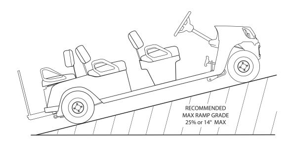
Fig. 3 Vechicle Dimensions, Incline Specifications
