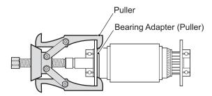
Fig. 9 Bearing Removal
