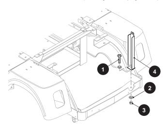
Fig. 18 Rear Bed Bracket Removal
