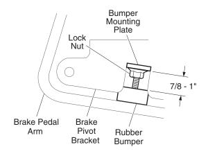
Fig. 3 Brake Pedal Bumper Adjustment
