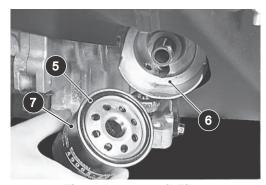
Fig. 7 Inspect Oil Filter
