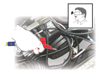
Fig. 16 Cleaning Cooling System with Air
