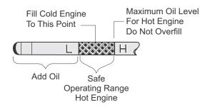
Fig. 2 Check Oil Level on Dipstick
