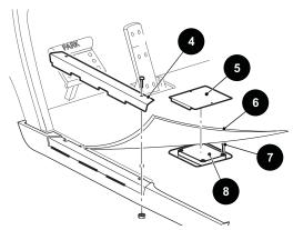
Fig. 4 Pedal Box Access
