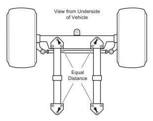
Fig. 8 Front Axle Alignment
