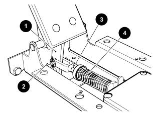
Fig. 8 Accelerator Pedal Arm Adjustment
