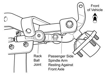
Fig. 20 Spindle Contact with Front Axle
