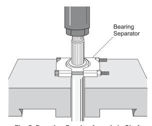
Fig. 5 Pressing Bearing from Axle Shaft
