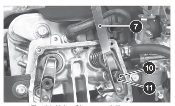
Fig. 21 Valve Clearance Adjustment
