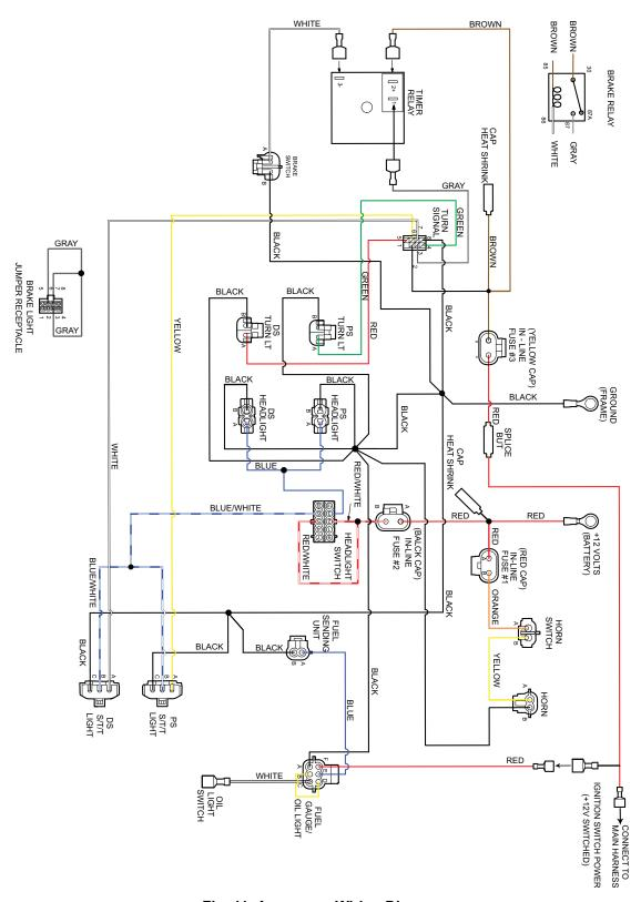
Fig. 11 Accessory Wiring Diagram
