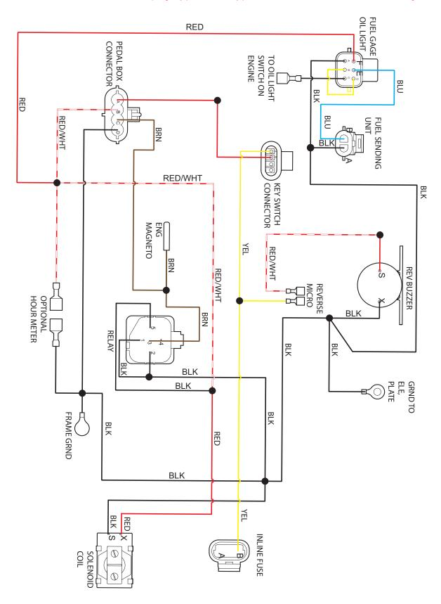
Fig. 1 Electrical System Wiring Diagram
