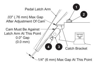
Fig. 27 Catch Bracket and Latch Arm Parking Brake Pedal, Removal and Installation
