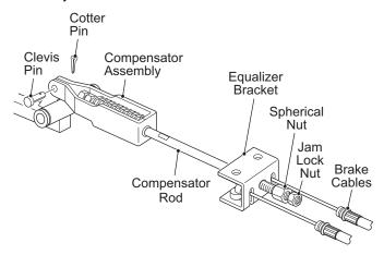
Fig. 25 Brake Cable, Equalizer and Compensator
