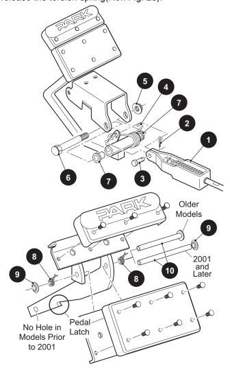
Fig. 26 Brake Pedal Removal and Installation.
