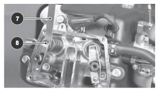
Fig. 20 Measure Valve Clearance
