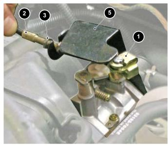
Fig. 4 Choke Cable and Housing
