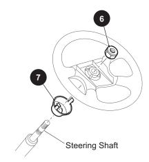
Fig. 23 Steering Wheel Replacement
