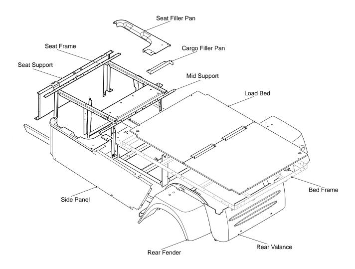
Fig. 5 Shuttle 2 Rear Body
