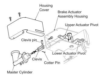
Fig. 1 Master Cylinder Replacement.
