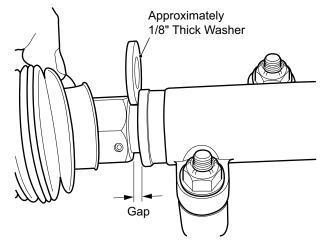
Fig. 21 Checking Gap
