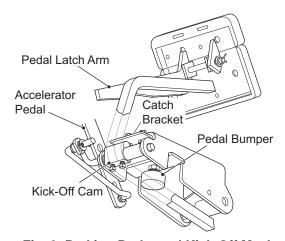
Fig. 3 Parking Brake and Kick-Off Mechanism
