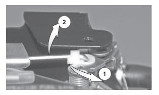
Fig. 6 Throttle Rod Removal
