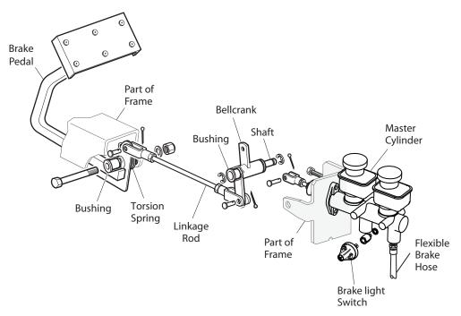
Fig. 1 Hydraulic Brake system Components
