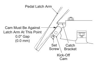
Fig. 11 Kick-off Cam Inspection
