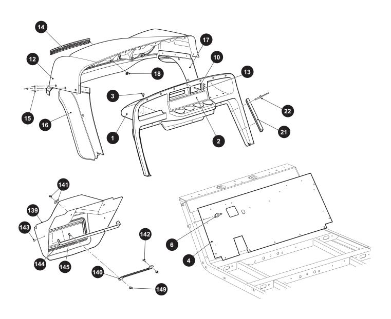
Fig. 2 Body Components Front
