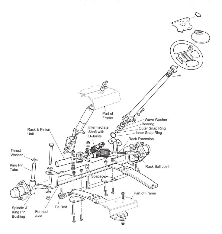
Fig. 1 Axle Mounted Steering and Front Suspension
