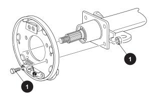
Fig. 22 Backing Plate Removal and Installation
