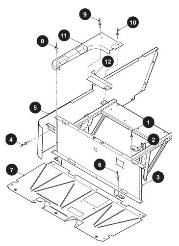
Fig. 8 Seat Support Removal
