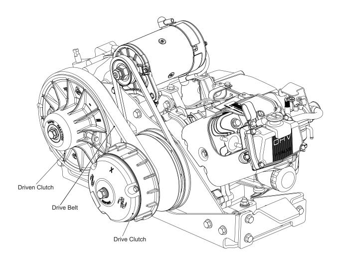
Fig. 1 Continuously Variable Transmission System (CVT)
