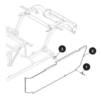
Fig. 11 Side Panel Removal
