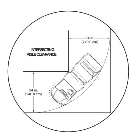
Fig. 4 Turning Clearance Diameter
