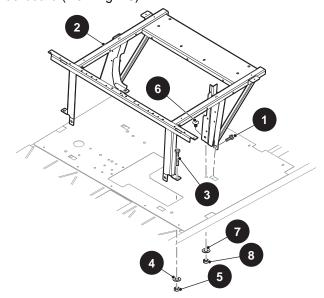
Fig. 16 Seat Frame Removal
