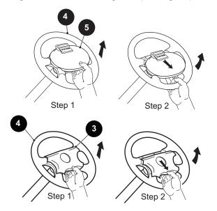
Fig. 22 Clipboard or Steering Wheel Cover Removal
