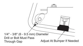
Fig. 6 Brake Pedal Bumper Inspection
