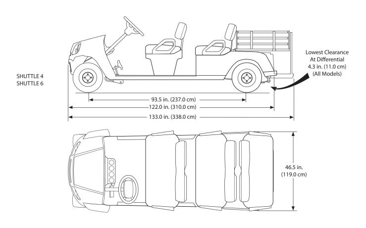
Fig. 1 Vechicle Dimensions (Shuttle 4 and 6)
