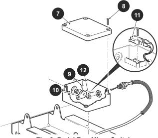
Fig. 9 Pedal Box Micro Switch
