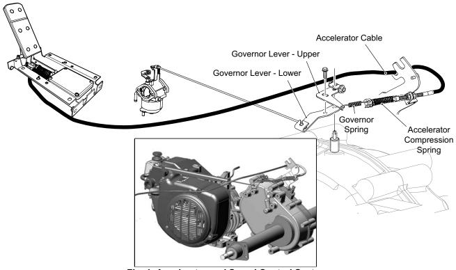
Fig. 1 Accelerator and Speed Control System
