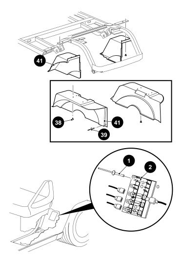
Fig. 9 Rear Fender Removal
