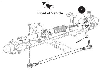
Fig. 2 Lubrication Points
