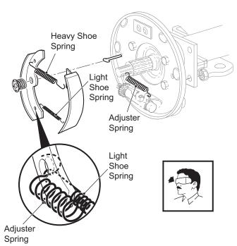
Fig. 16 Orientation of Brake Shoe Springs
