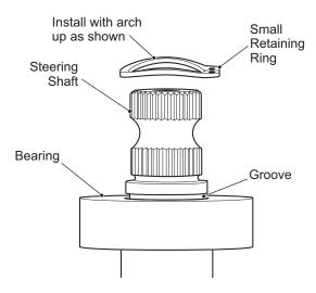
Fig. 25 Small Retaining Ring Orientation
