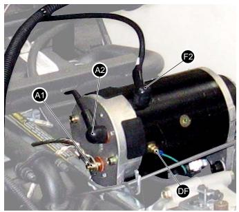
Fig. 14 Starter/Generator Wire Connections
