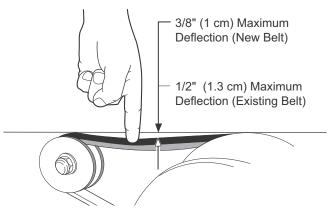
Fig. 11 Checking Belt Tension with Finger
