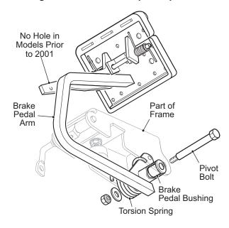
Fig. 7 Brake Pedal Inspection
