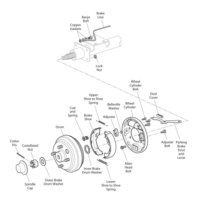
Fig. 5 Wheel Brake Components
