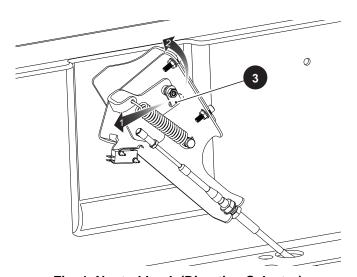
Fig. 1 Neutral Lock (Direction Selector)
