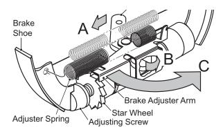
Fig. 2 Wheel Brake Adjustment
