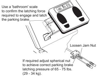
Fig. 19 Checking Parking Brake Latching Pressure
