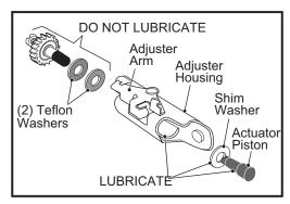
Fig. 21 Wheel Brake Lubrication Points
