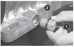
Fig. 5 Oil Drain Plug
