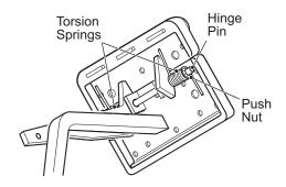
Fig. 10 Parking Brake Pedal Hinge Inspection
