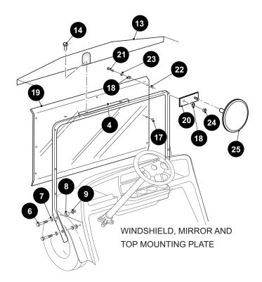
Fig. 1 Front Strut, Windshield and Mirror Installation
