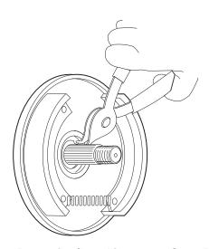
Fig. 3 Removing/Installing Outer Snap Ring
