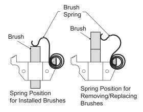
Fig. 8 Starter/Generator Brush Removal
