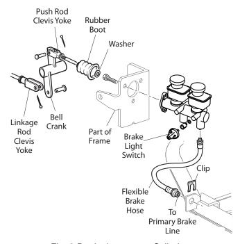
Fig. 2 Replacing master Cylinder
