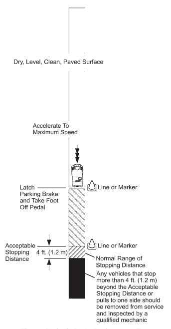
Fig. 12 Periodic Brake Performance Test
