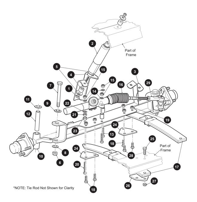
Fig. 6 Front Suspension Components
