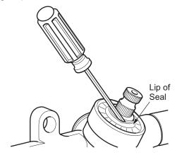
Fig. 16 Pinion Seal Replacement
