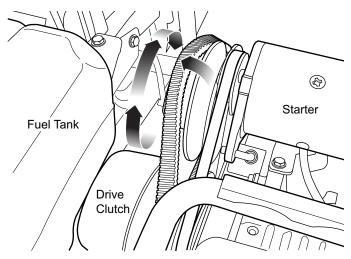
Fig. 2 Removing the Drive Belt
