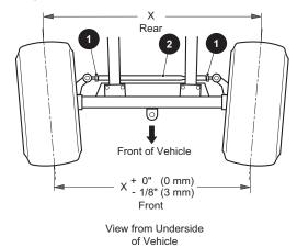
Fig. 4 Wheel Alignment
