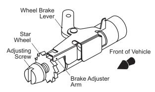
Fig. 14 Adjuster Mechanism
