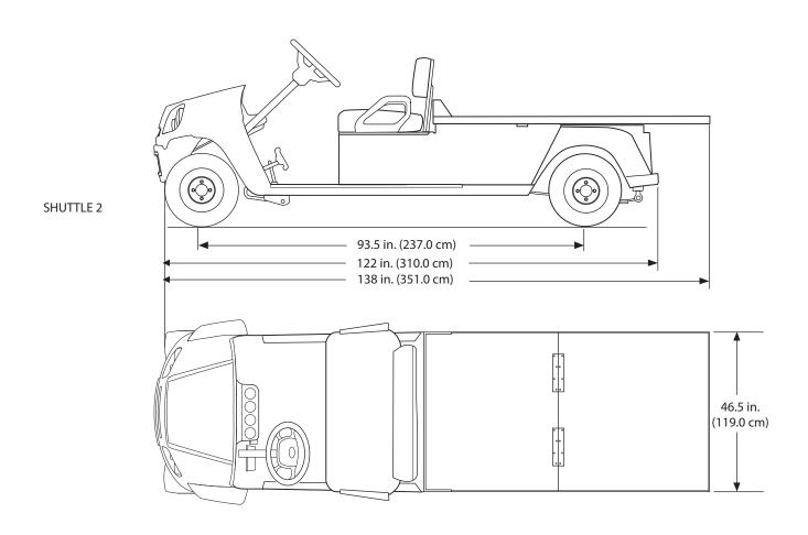
Fig. 2 Vechicle Dimensions (Shuttle 2)
