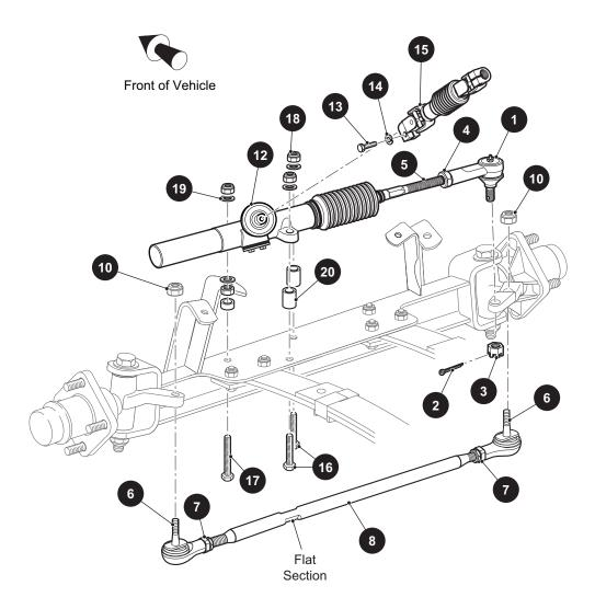
Fig. 12 Steering Components
