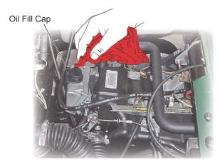
Fig. 4 Cleaning Top of Engine
