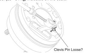
Fig. 18 Check Clevis Pins.
