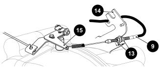
Fig. 3 Accelerator Cable at Governor
