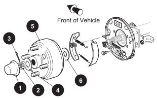
Fig. 20 Brake Assembly
