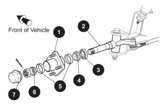
Fig. 11 Wheel Bearing Replacement
