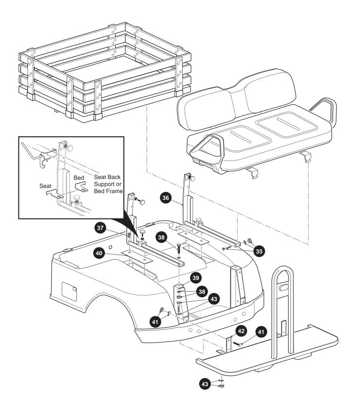
Fig. 4 Body Components (Cargo Box, Seat, Foot Rest)
