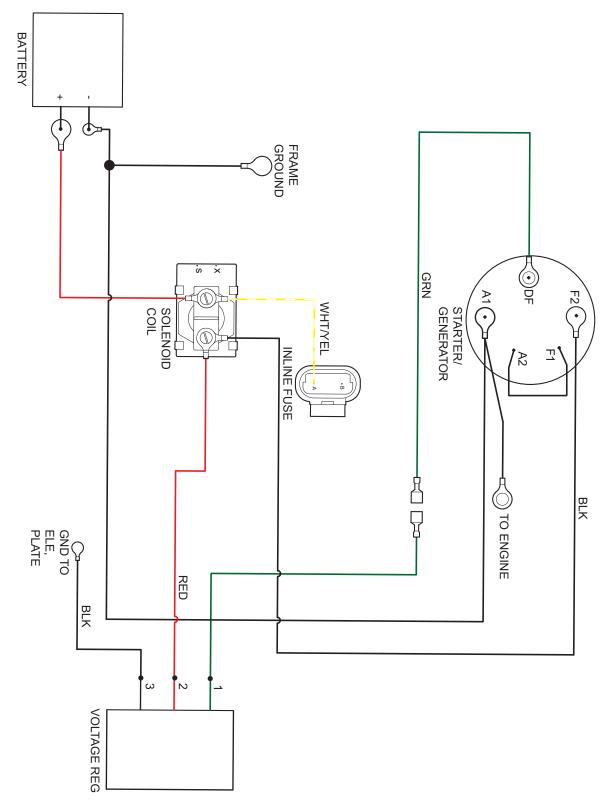
Fig. 2 Electrical System Wiring Diagram
