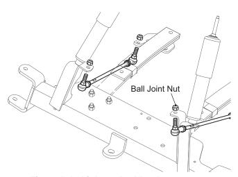
Fig. 7 Axle Linkage Rod Replacement
