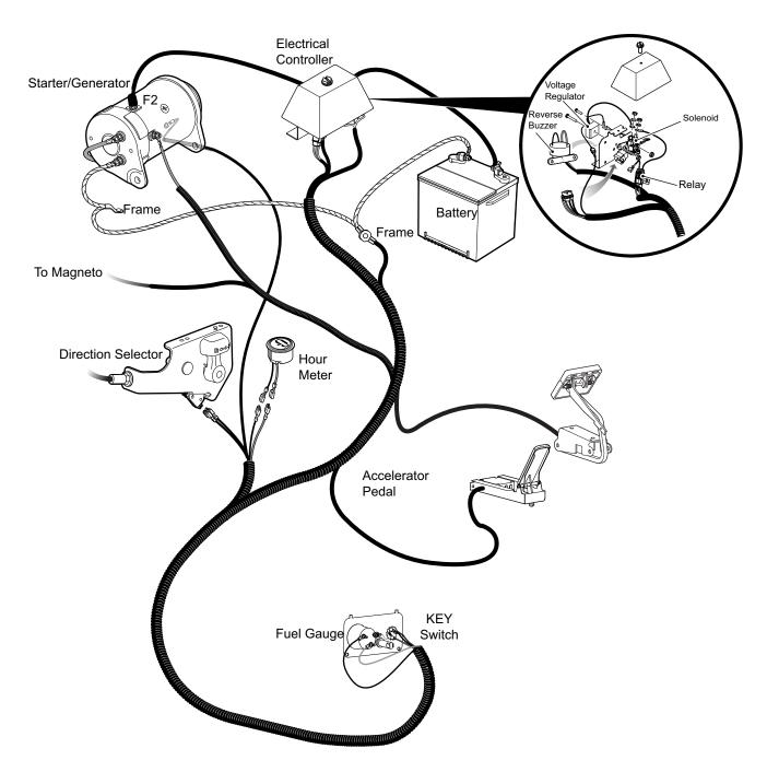
Fig. 3 Electrical System (Physical Location)
