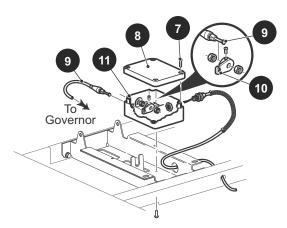
Fig. 5 Accelerator Cable at Pedal Box
