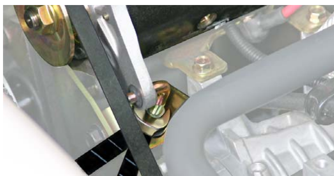
Fig. 13 Adjusting the Belt Tension
