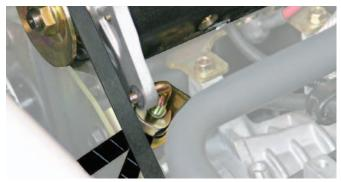
Fig. 13 Adjusting the Belt Tension
