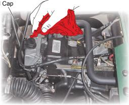
Fig. 4 Cleaning Top of Engine
