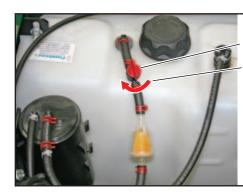
Fuel Shut-off Valve Turn to "OFF" Position
