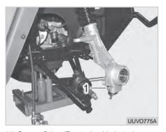
(1) Grease fitting (Front wheel hubstrut)
