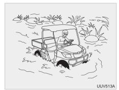
This vehicle can go through water as high as the floor of the vehicle.
