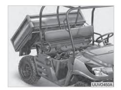
It is possible to inspect the engine for most items by removing the seat cushion and raising the cargo bed. For engine oil level check, just remove the inspection shield on the lower section of the seat.
