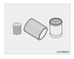
The various filters and air cleaner are consumables to filter foreign materials from oil and air. Make sure to check or replace these parts when changing oil.
