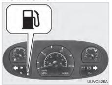
This lamp comes on when the fuel tank is approaching empty. When it comes on, you should add fuel as soon as possible. Driving with the this lamp on or with the fuel level below "E" can cause the engine to misfire and damage the engine parts.
