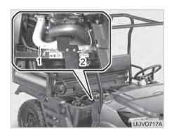
(1) Heat shield cover 1 (2) Heat shield cover 2
