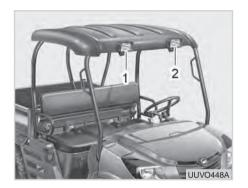
(1) Front Working Lamp (RH) (2) Front Working Lamp (LH)
