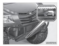
(1) Coolant Drain Plug Of Radiator
