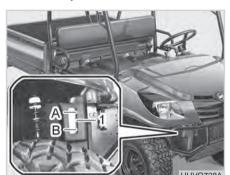
(1) Auxiliary coolant tank (A) MAX limit (B) MIN limit
