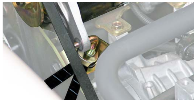
Fig. 13 Adjusting the Belt Tension
