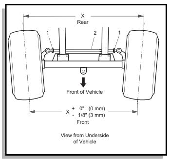
Fig. 4 Wheel Alignment
