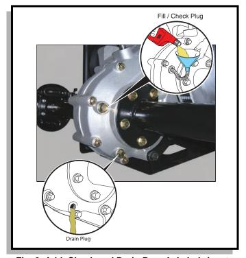
Fig. 2 Add, Check and Drain Rear Axle Lubricant
