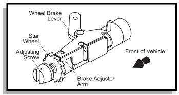
Fig. 15 Adjuster Mechanism
