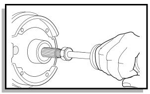
Fig. 4 Removing/Installing Axle Shaft
