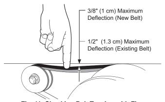
Fig. 11 Checking Belt Tension with Finger
