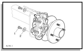
Fig. 16 Removing Brake Caliper
