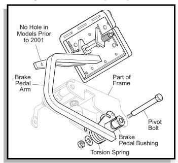
Fig. 8 Brake Pedal Inspection
