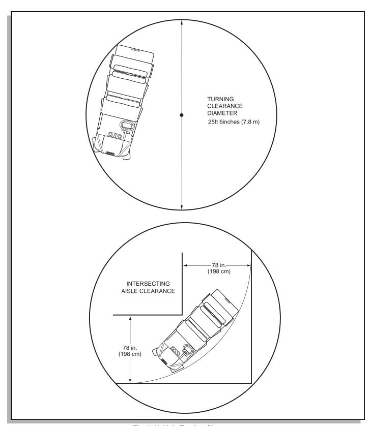
Fig. 3 Vehicle Turning Clearance
