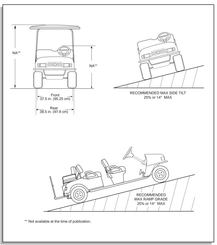
Fig. 2 Vehicle Dimensions and incline Specifications
