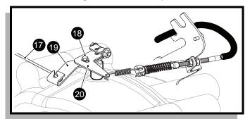
Fig. 7 Throttle Rod Adjustment
