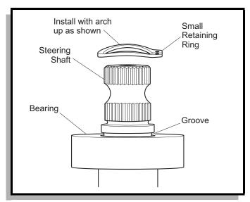
Fig. 24 Small Retaining Ring Orientation
