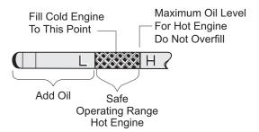
Fig. 2 Check Oil Level on Dipstick
