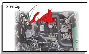
Fig. 4 Cleaning Top of Engine
