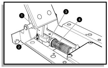
Fig. 8 Accelerator Pedal Arm Adjustment
