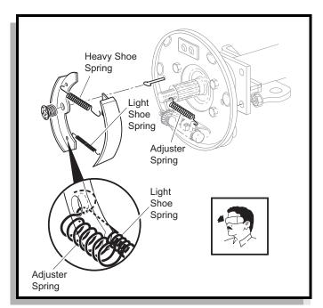
Fig. 17 Orientation of Brake Shoe Springs
