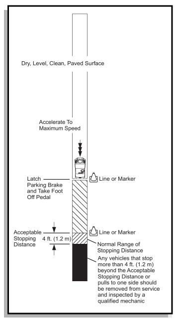
Fig. 13 Periodic Brake Performance Test
