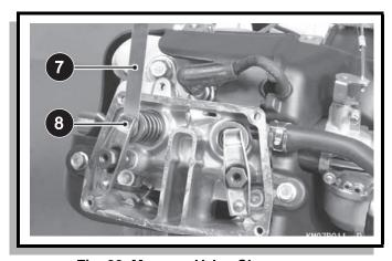
Fig. 20 Measure Valve Clearanvce
