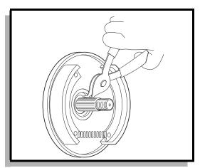
Fig. 3 Removing/Installing Outer Snap Ring
