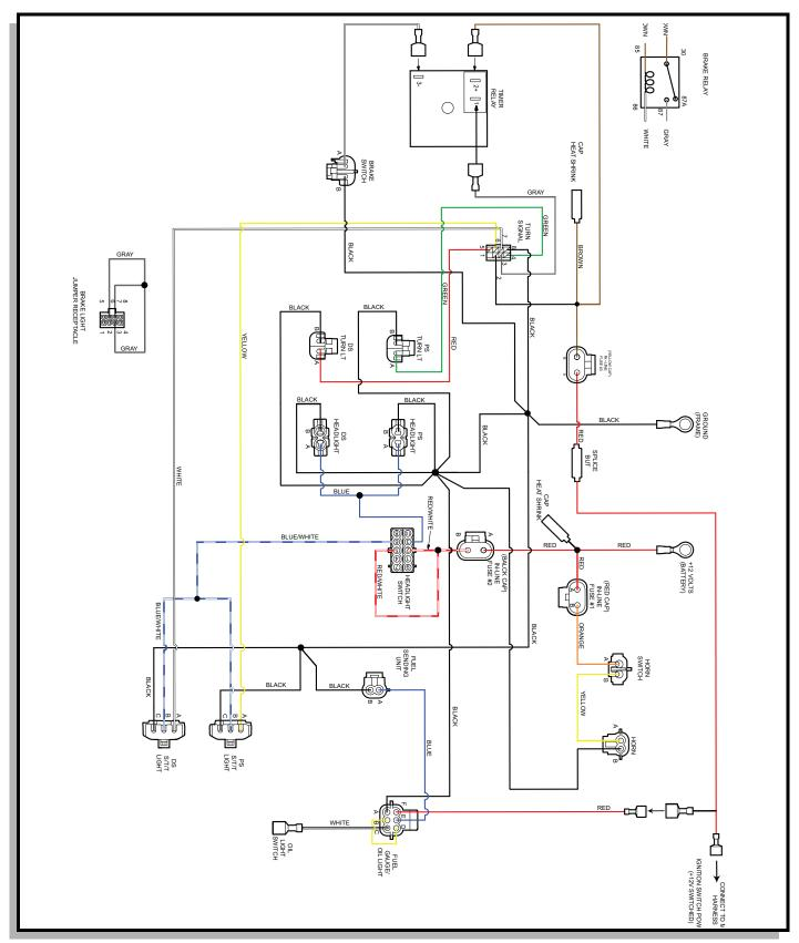
Fig. 11 Accessory Wiring Diagram
