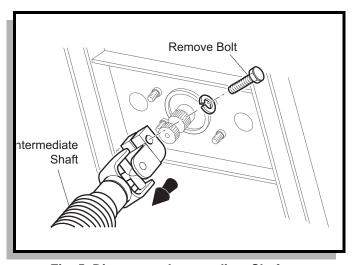
Fig. 5 Disconnect Intermediate Shaft to Center Steering Wheel
