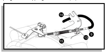
Fig. 3 Accelerator Cable At Governor
