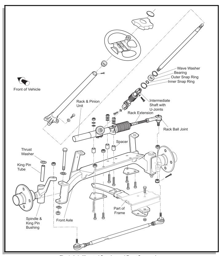
Fig. 1 Axle Mounted Steering and Front Suspension
