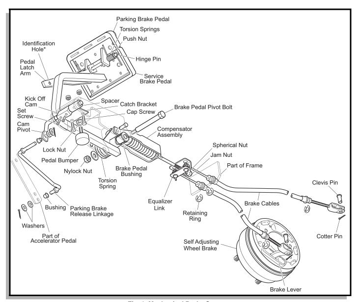
Fig. 1 Mechanical Brake System
