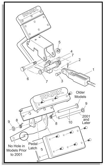
Fig. 27 Brake Pedal Removal and Installation
