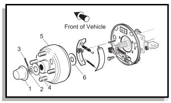
Fig. 21 Brake Assembly
