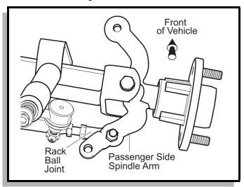
Fig. 19 Spindle Contact with Front Axle
