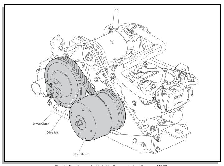
Fig. 1 Continuously Variable Transmission System (CVT)
