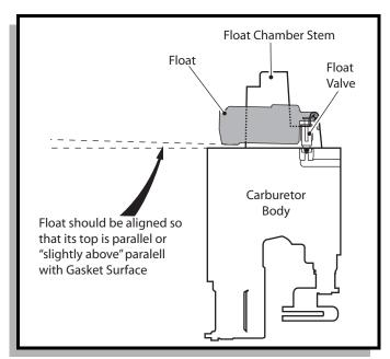
Fig. 7 Float Adjustment
