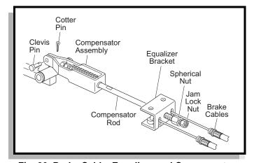
**Fig. 26** Brake Cable, Equalizer and Compensator Adjust the brake pedal free travel. "Adjusting Brake Pedal Free Travel" on page M 14
