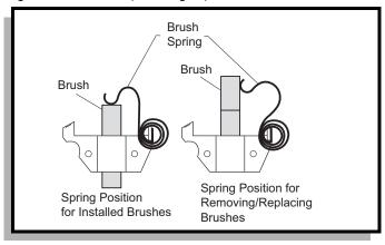
Fig. 8 Starter/Generator Brush Removal
