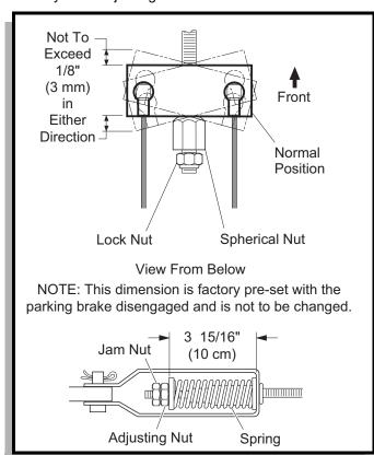
Fig. 10 Equalizer and Compensator
