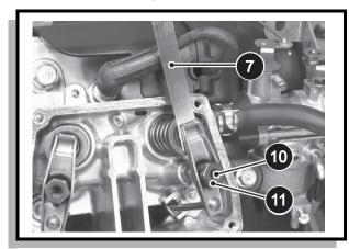
Fig. 21 Valve Clearance Adjustment
