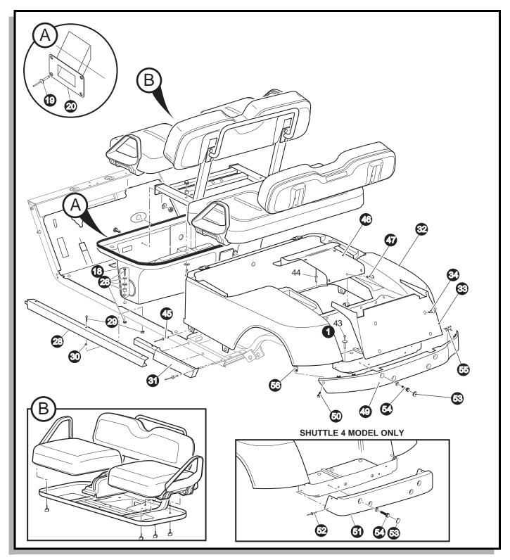
Fig. 3 Body Components (Seats and Rear)
