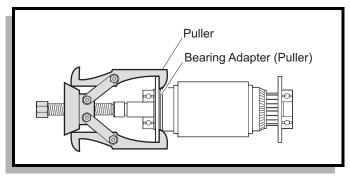
Fig. 9 Bearing Removal
