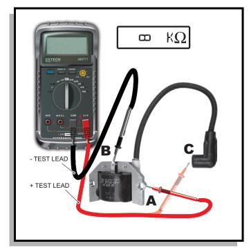
Fig. 5 Resistance Between B - A and B - C
