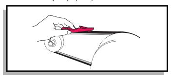
Fig. 10 Checking Belt Tension with Gauge
