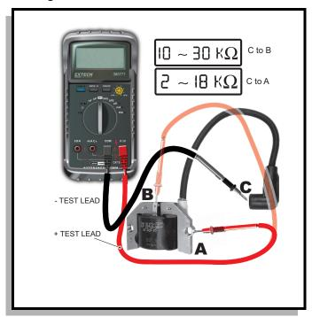
Fig. 6 Resistance Between C - B and C - A
