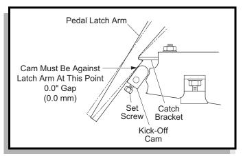
Fig. 28 Catch Bracket and Latch Arm
