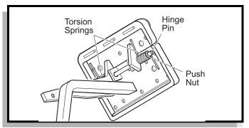
Fig. 11 Parking Brake Pedal Hinge Inspection
