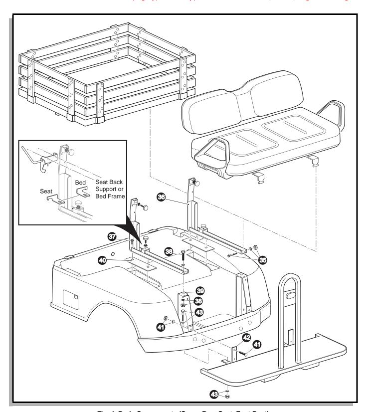
Fig. 4 Body Components (Cargo Box, Seat, Foot Rest)
