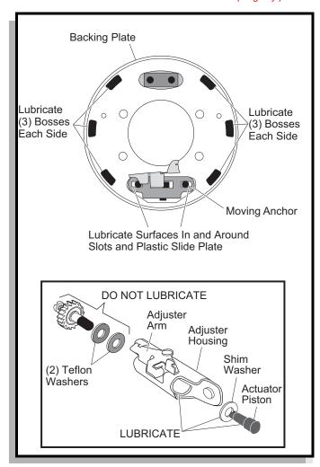
Fig. 22 Wheel Brake Lubrication Points
