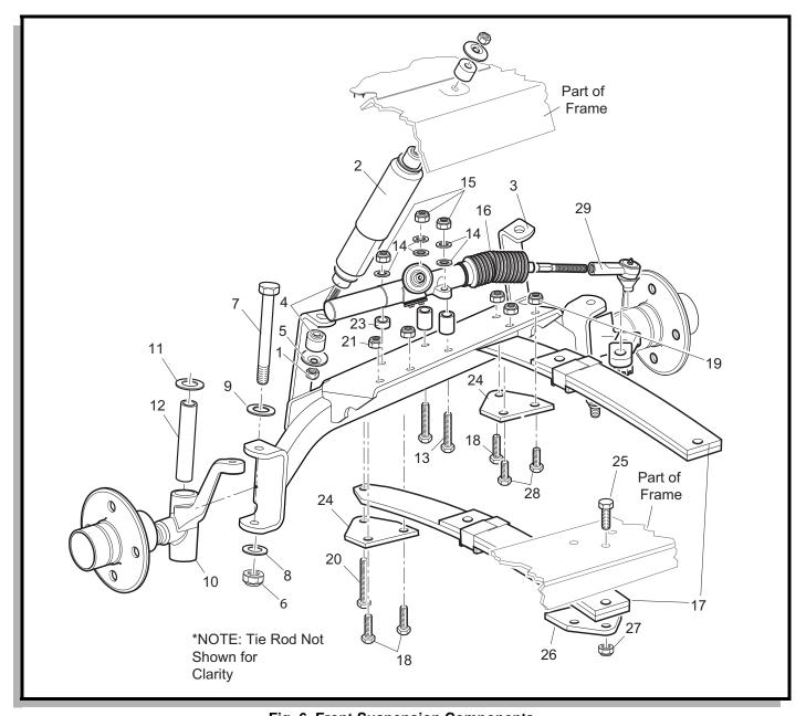
Fig. 6 Front Suspension Components
