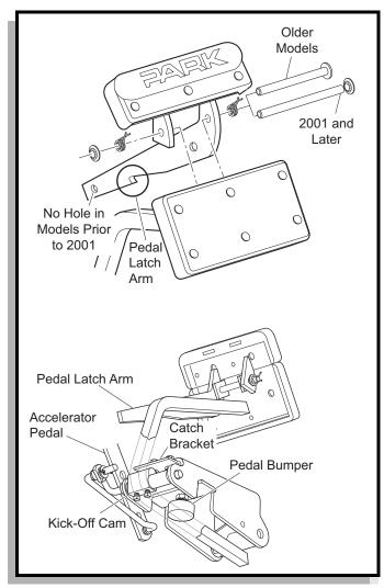
Fig. 3 Parking Brake and Kick-Off Mechanism
