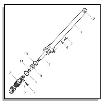
Fig. 23 Steering Shaft and Column
