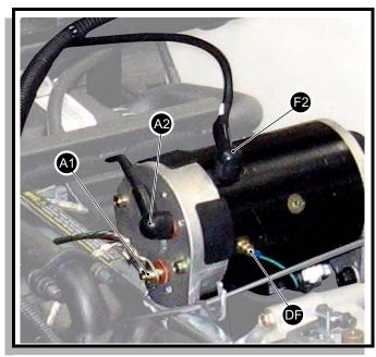
Fig. 14 Starter/Generator Wire Connections
