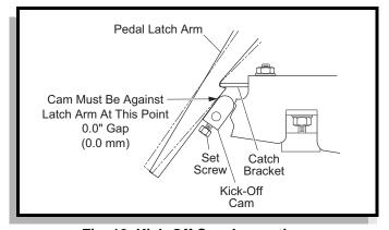
Fig. 12 Kick-Off Cam Inspection
