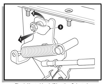
Fig. 1 Neutral Lock (Direction Selector)
