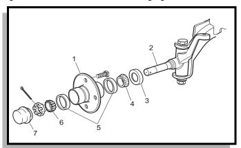
Fig. 10 Wheel Bearing Replacement
