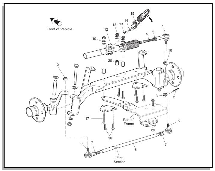
Fig. 11 Steering Components
