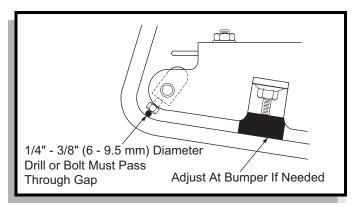
Fig. 7 Brake Pedal Bumper Inspection
