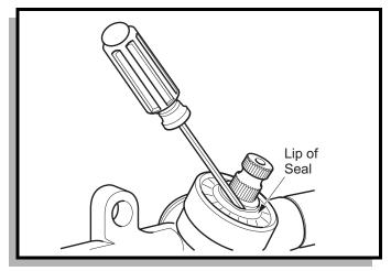
Fig. 15 Pinion Seal Replacement
