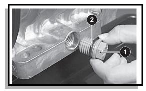
Fig. 5 Oil Drain Plug
