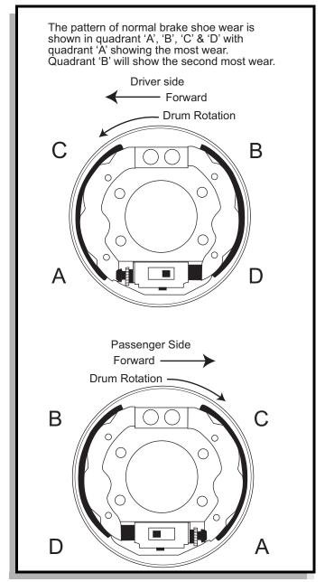
Fig. 16 Brake Shoe Wear
