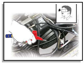
Fig. 16 Cleaning Cooling System With Air
