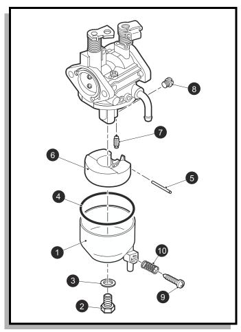
Fig. 6 Carburetor Disassembly
