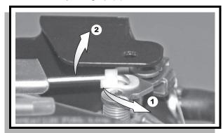
Fig. 6 Throttle Rod Removal
