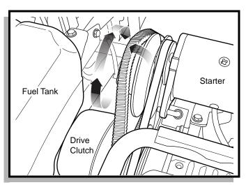
Fig. 2 Removing the Drive Belt
