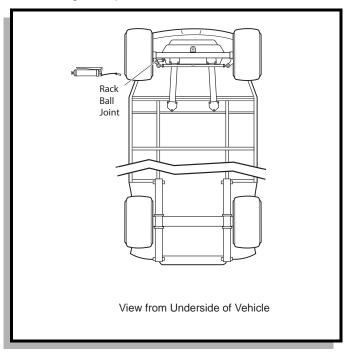
Fig. 5 .Lubrication Points
