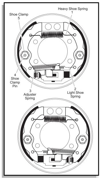
Fig. 24 Brake Shoes and Springs
