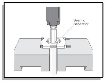
Fig. 5 Pressing Bearing from Axle Shaft
