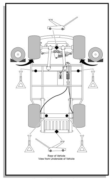
Fig. 2 Lifting the vehicle
