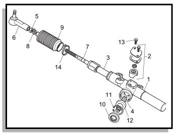
Fig. 18 Rack and Pinion Unit Disassembly
