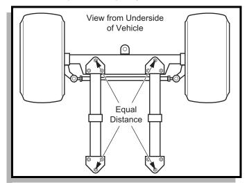
Fig. 7 Front Axle Alignment
