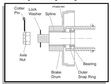
Fig. 7 Cut Away of Outer Bearing and Brake Drum
