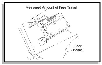
Fig. 9 Checking for Excessive Free Travel
