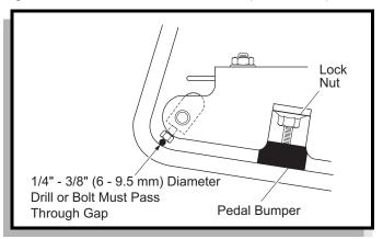
Fig. 29 Pedal Bumper Adjustment
