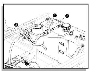
Fig. 9 Fuel Lines And Filter
