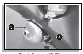
Fig. 6 Remove Oil Filter
