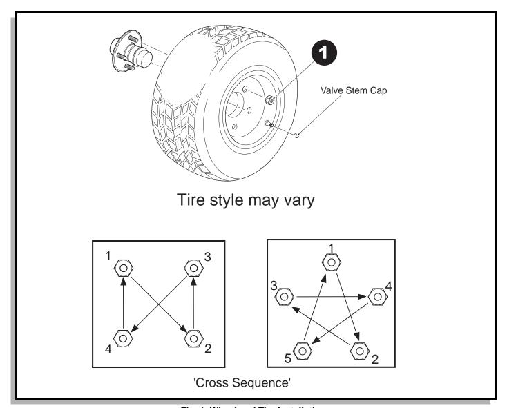
Fig. 1 Wheel and Tire Installation
