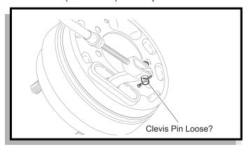
Fig. 19 Check Clevis Pins
