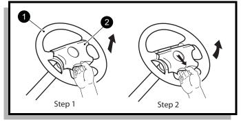
Fig. 21 Steering Wheel Cover Removal
