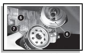
Fig. 7 Inspect Oil Filter
