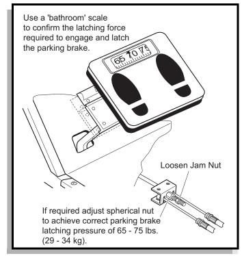
Fig. 20 Checking Parking Brake Latching Pressure
