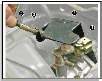
Fig. 4 Choke Cable And Housing
