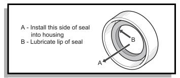
Fig. 9 Seal Installation
