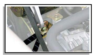
Fig. 13 Adjusting Belt Tension
