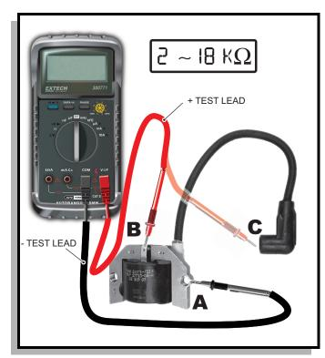
Fig. 4 Resistance Between A - B and A - C
