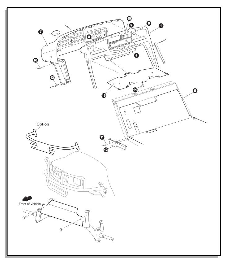
Fig. 2 Body Components (Front)
