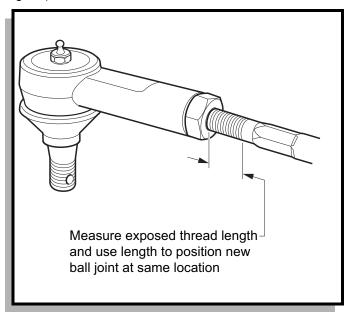
Fig. 12 Rack Ball Joint Installation
