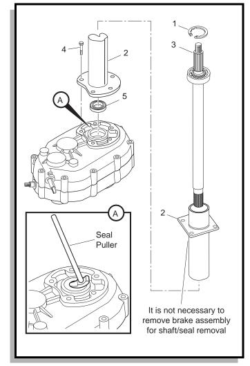
Fig. 6 Removing/Installing Seal
