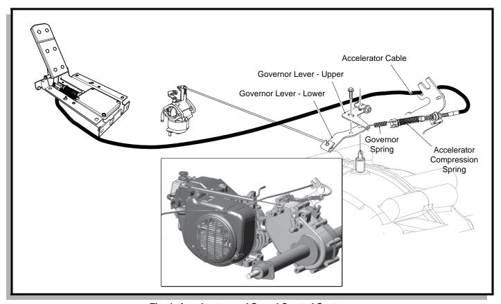
Fig. 1 Accelerator and Speed Control System
