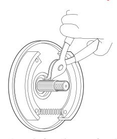
Fig. 3 Removing/Installing Outer Snap Ring
