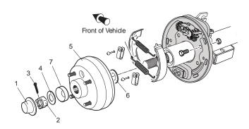
Fig. 21 Brake Assembly
