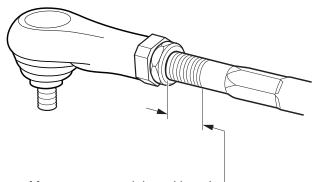
Measure exposed thread length and use length to position new ball joint at same location
