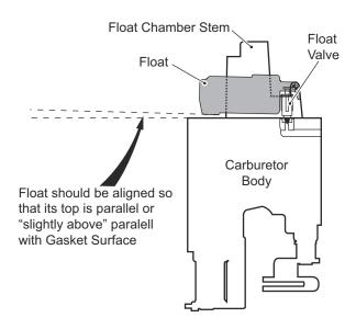
Fig. 7 Float Adjustment
