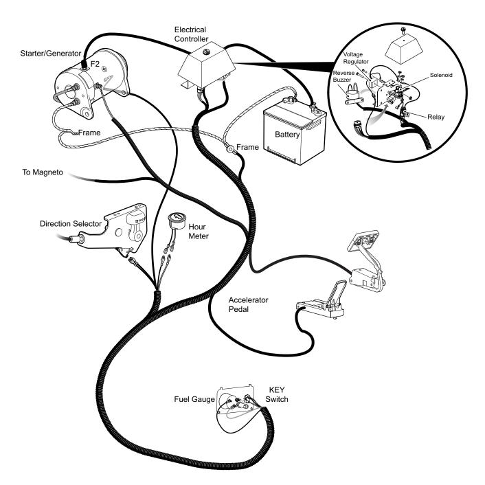
Fig. 3 Electrical System (Physical Location)
