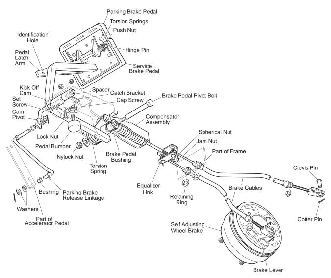
Fig. 1 Mechanical Brake System
