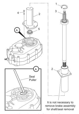
Fig. 6 Removing/Installing Seal
