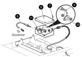
Fig. 5 Accelerator Cable at Pedal Box
