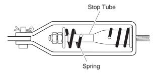
Fig. 3 Compensator Assembly
