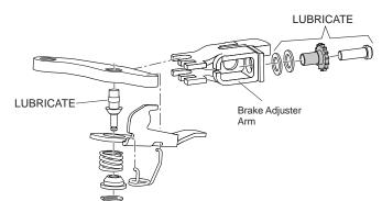
Fig. 22 Wheel Brake Lubrication Points
