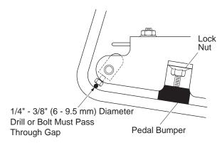
Fig. 30 Pedal Bumper Adjustment
