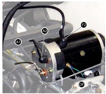
Fig. 14 Starter/Generator Wire Connections
