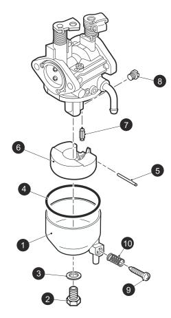
Fig. 6 Carburetor Disassembly
