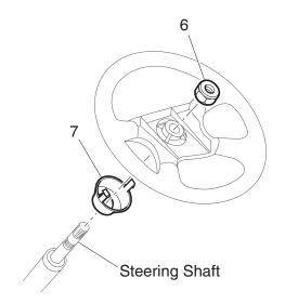
Fig. 21 Steering Wheel Replacement
