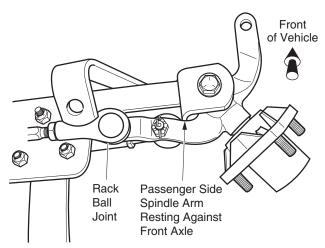
Fig. 18 Spindle Contact with Front Axle
