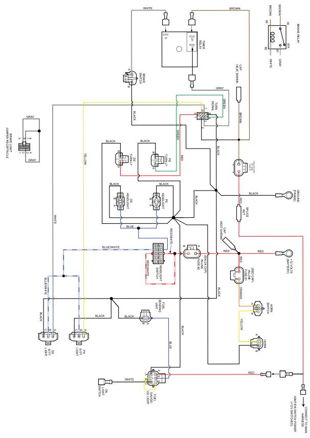
Fig. 11 Accessory Wiring Diagram
