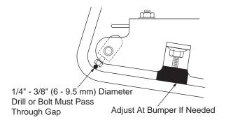
Fig. 7 Brake Pedal Bumper Inspection
