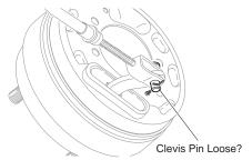
Fig. 19 Check Clevis Pins
