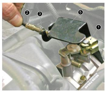
Fig. 4 Choke Cable and Housing
