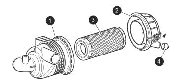
Fig. 9 Air Filter Assembly
