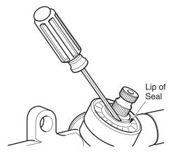
Fig. 15 Pinion Seal Replacement
