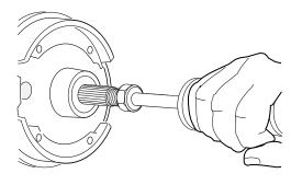
Fig. 4 Removing/Installing Axle Shaft
