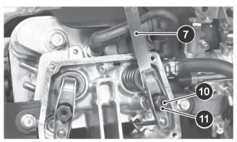
Fig. 21 Valve Clearance Adjustment
