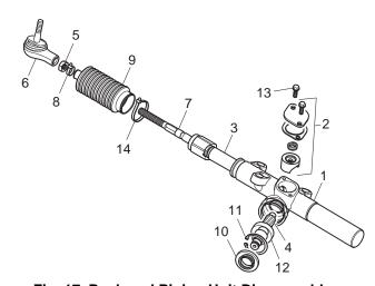
Fig. 17 Rack and Pinion Unit Disassembly
