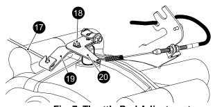
Fig. 7 Throttle Rod Adjustment
