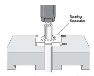
Fig. 5 Pressing Bearing from Axle Shaft
