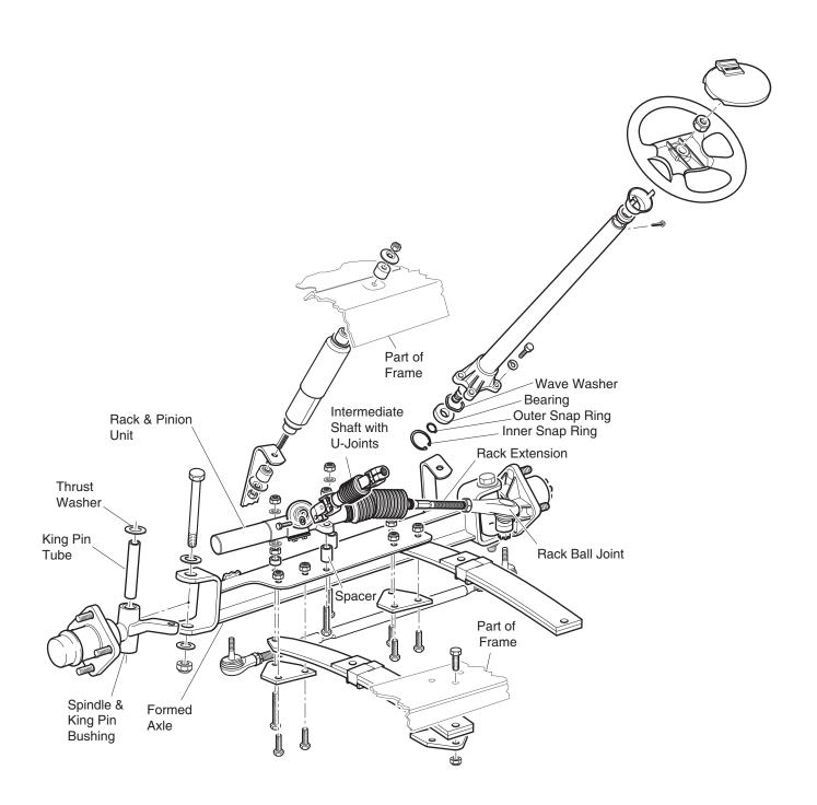
Fig. 1 Steering and Front Suspension
