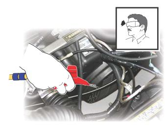
Fig. 16 Cleaning Cooling System with Air
