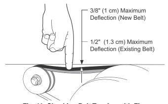
Fig. 11 Checking Belt Tension with Finger
