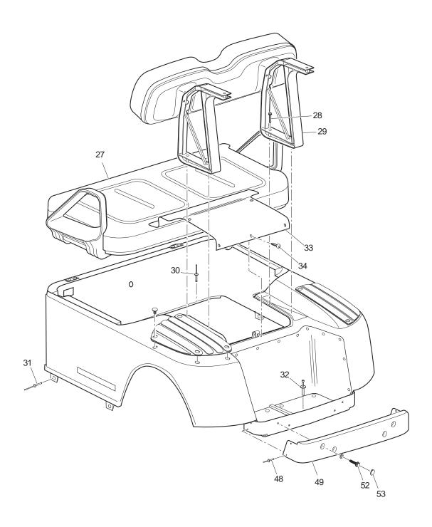
Fig. 3 Body Components (Rear)
