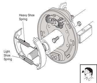
Fig. 17 Orientation of Brake Shoe Springs
