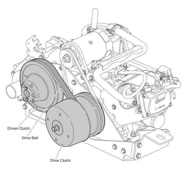
Fig. 1 Continuously Variable Transmission System (CVT)
