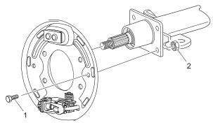
Fig. 23 Backing Plate Removal and Installation
