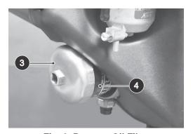
Fig. 6 Remove Oil Filter
