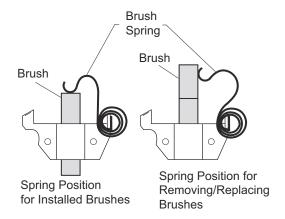
Fig. 8 Starter/Generator Brush Removal
