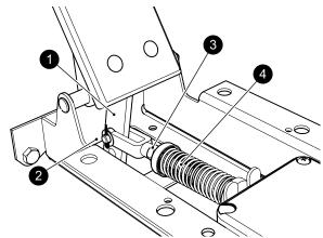
Fig. 8 Accelerator Pedal Arm Adjustment
