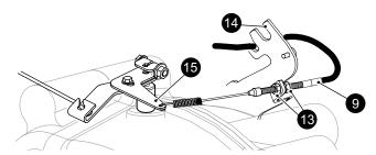
Fig. 3 Accelerator Cable at Governor
