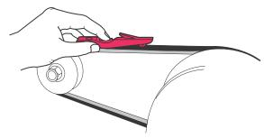
Fig. 10 Checking Belt Tension with Gauge
