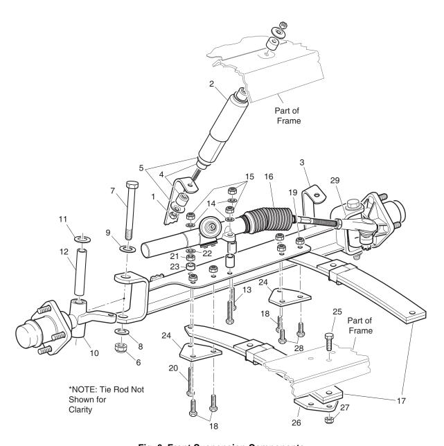
Fig. 6 Front Suspension Components
