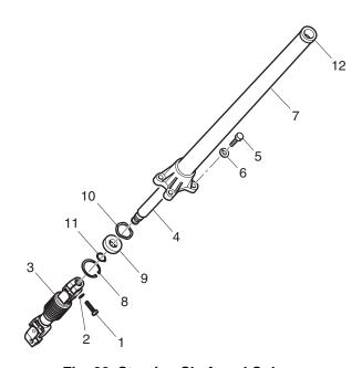
Fig. 22 Steering Shaft and Column
