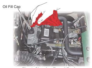
Fig. 4 Cleaning Top of Engine
