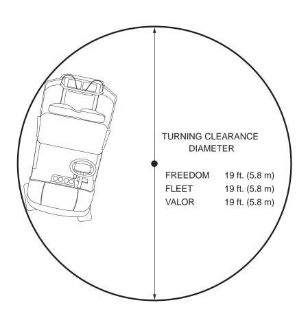
Fig. 2 Vehicle Turning Clearance
