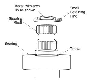
Fig. 23 Small Retaining Ring Orientation
