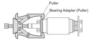
Fig. 9 Bearing Removal
