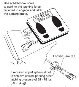
Fig. 20 Checking Parking Brake Latching Pressure
