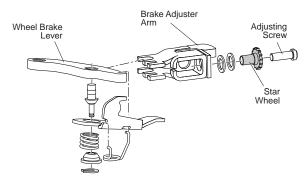
Fig. 15 Adjuster Mechanism
