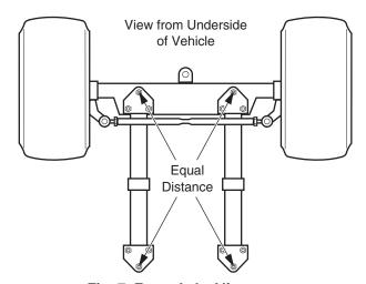
Fig. 7 Front Axle Alignment
