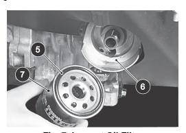
Fig. 7 Inspect Oil Filter
