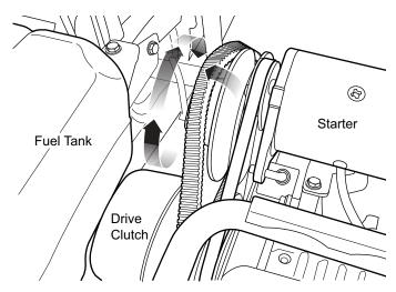
Fig. 2 Removing the Drive Belt
