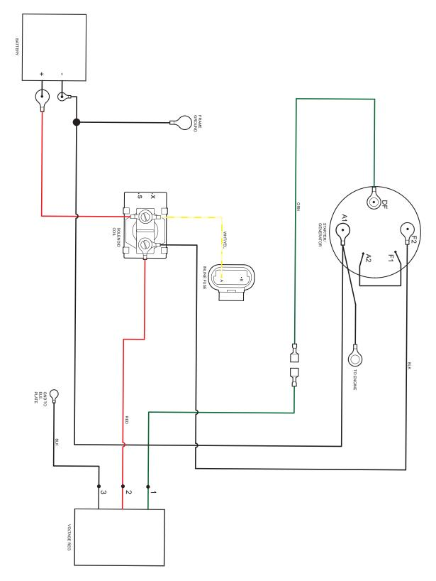
Fig. 2 Electrical System Wiring Diagram
