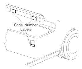
Fig. 1 Serial Number Plate & Location
