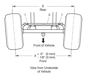
Fig. 4 Wheel Alignment
