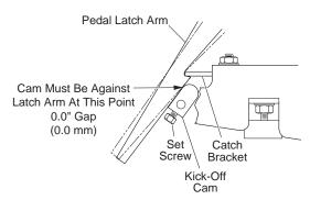
Fig. 12 Kick-Off Cam Inspection
