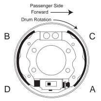
Fig. 16 Brake Shoe Wear
