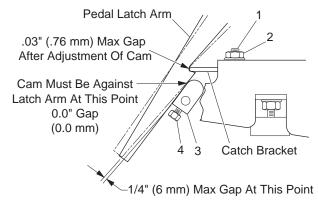
Fig. 29 Catch Bracket and Latch Arm Parking Brake Pedal Removal and Installation
