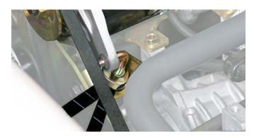
Fig. 13 Adjusting the Belt Tension
