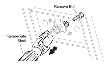
Fig. 5 Disconnect Intermediate Shaft to Center Steering Wheel
