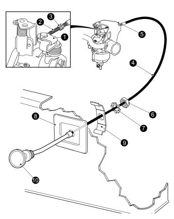
Fig. 3 Choke Cable Attachment
