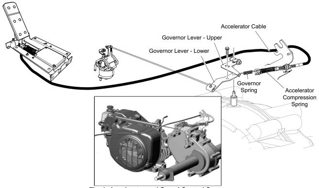
Fig. 1 Accelerator and Speed Control System
