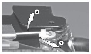
Fig. 6 Throttle Rod Removal
