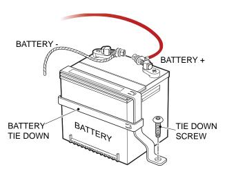
Fig. 1 Battery Removal
