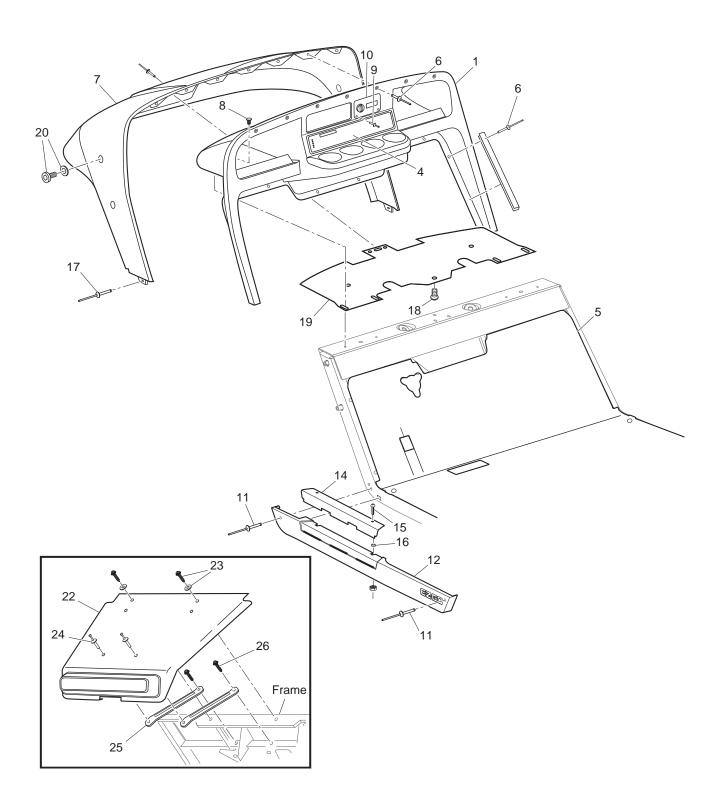
Fig. 2 Body Components (Front)
