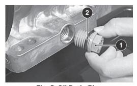
Fig. 5 Oil Drain Plug
