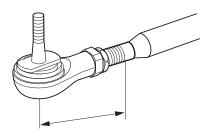
Measure distance from center of ball joint to jam nut and use length to position new ball joint at same location
