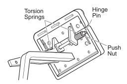
Fig. 11 Parking Brake Pedal Hinge Inspection
