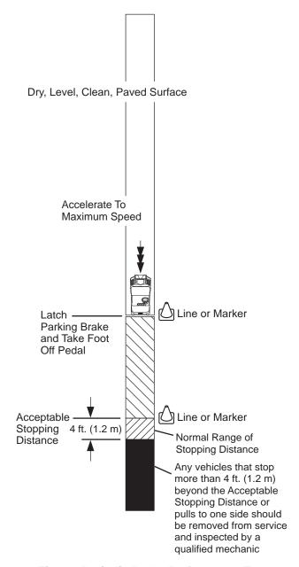
Fig. 13 Periodic Brake Performance Test
