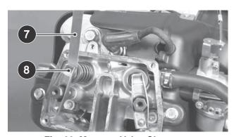
Fig. 20 Measure Valve Clearance
