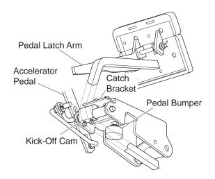
Fig. 2 Parking Brake and Kick-Off Mechanism
