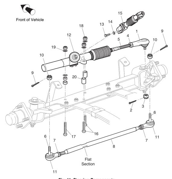
Fig. 11 Steering Components
