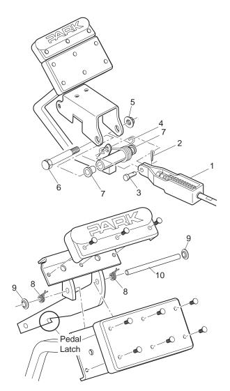
Fig. 28 Brake Pedal Removal and Installation
