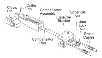
Fig. 26 Brake Cable, Equaliser and Compensator
