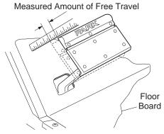
Fig. 9 Check for Excessive Free Travel
