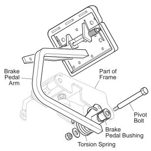
Fig. 8 Brake Pedal Inspection
