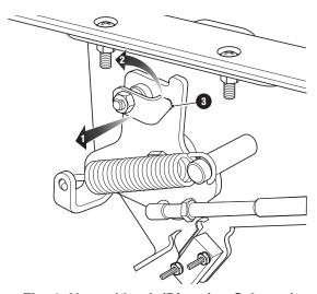
Fig. 1 Neutral Lock (Direction Selector)
