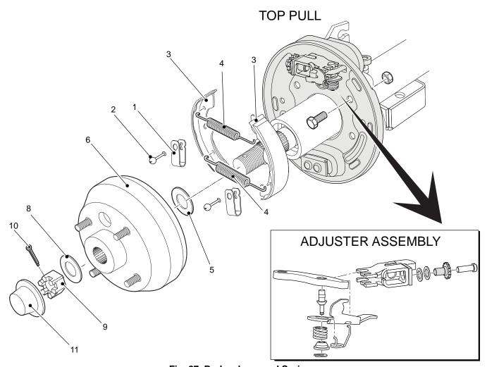
Fig. 27 Brake shoes and Springs
