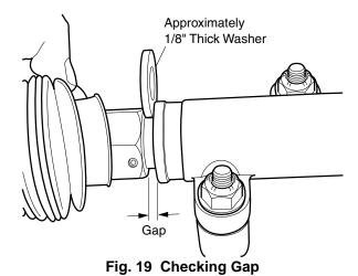
Adjust, using an 1/8" thick washer as a gauge, by turning shaft of rack extension with wrench to create the 1/8" gap. Tighten jam nut (5) to 35 - 45 ft. lbs. (47 - 61 Nm) torque. Secure bellows to rack and pinion unit with new wire tie (14).
