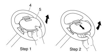
Fig. 20 Clipboard Removal
