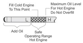
Fig. 2 Check Oil Level on Dipstick
