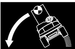
LOAD WITH HIGH CENTER OF GRAVITY COULD RESULT IN TIP OVER
