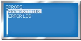
Past 7 Error Codes are displayed on ERROR LOG screen. The error code along with the run time when the error occurred. This is past history and is not the current fault being experienced unless the L time and CPU time are very close to being equal.
