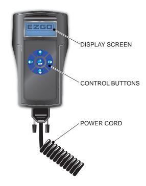
The vertical bar along the left side of the display screen moves up and down when buttons 1 or 5 are pressed. The length of the bar also changes depending on how many items are in a menu. When the bar is positioned at the top arrow the beginning of the menu has been reached; if the bar has reached the arrow at the bottom of the screen there are no more menu choices available.
