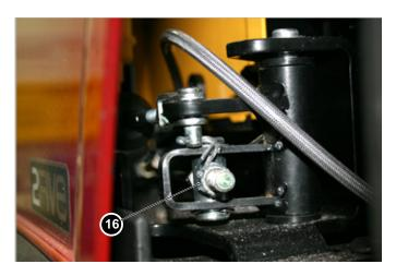
Fig. 4 Cable Adjusting Nut
