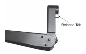
Fig. 10 Wiper Arm Release Tab
